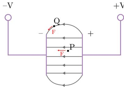
The electric field should be straight between the plates, from left to right, because a particle between the plates experiences a force directly to the negative plate. However, the lines should be curved around the edges because a charge on the edge will experience a force that is not horizontal.
