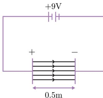
The positive terminal of the battery is on the left, so the left-hand plate will be positively charged, whereas the right terminal and plate are negatively charged. We draw electric field lines in the positive to negative direction.
