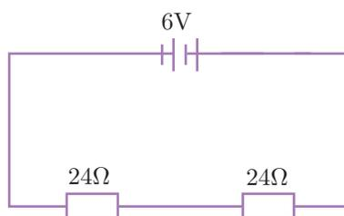
ii. This is a series circuit, so we use  $R_T = R_1 + R_2$  to calculate the total resistance, which is  $R_T = 24 + 24 = 48\Omega$ .
