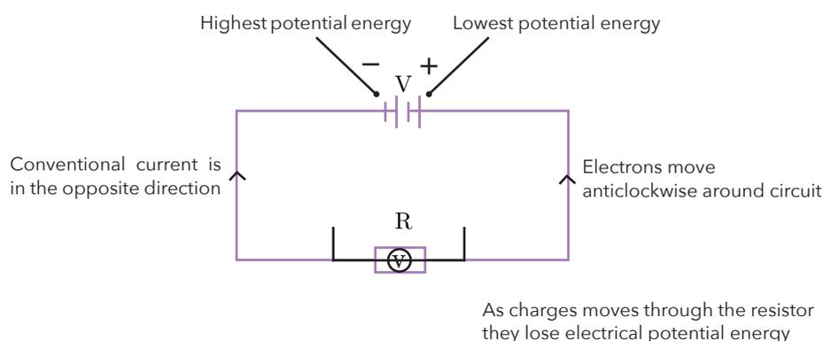
i. The electrons will move from high potential energy at the negative terminal to low potential energy at the positive terminal. This means that the electrons will be moving anticlockwise around this circuit.
