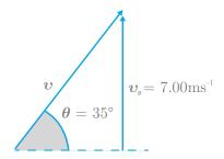
$$\begin{aligned} \tan(\theta) &= \frac{O}{A} = \frac{v_y}{v_x} \\ v_x &= \frac{v_y}{\tan(\theta)} \end{aligned}$$
