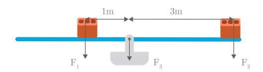
*ii.* An object is in rotational equilibrium when it has no net torques acting upon it. Since the seesaw is staying level, it is not rotating, which means that it has no net torques and is therefore in rotational equilibrium.
