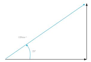
Drawing the horizontal and vertical vectors of the given velocity will help us figure out which trig formula we need to use.
