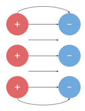
The direction of an electric field is shown by which way the arrows are pointing (which should always be from positive to negative charges). The strength of an electric field is shown by the number of lines in the diagram.
