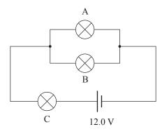
Calculate the total resistance of this circuit.
